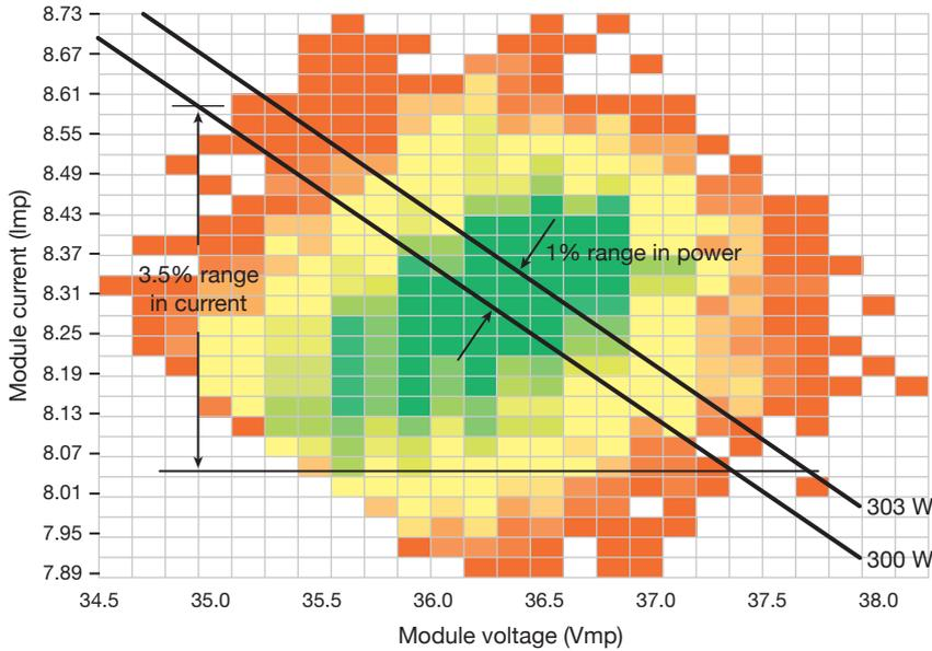
**Figure 1** Groups of modules with a 1% power tolerance can have a current tolerance of 3.5%. Think of the 3.5% current tolerance as the current-binning tolerance. Thus, a 1% power-binning tolerance does not reduce losses due to module mismatch as much as a 1% current-binning tolerance does.
