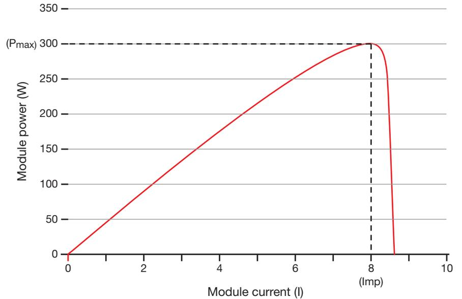
**Figure 3** This current versus power curve was derived from a standard c-Si module IV curve. Note that the curve is relatively flat near the peak power point, so small deviations in a module's operating current have very little effect on the module's power.
